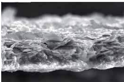
Illustration 1: REM of a zinc flake coat (20 \mu\text{m} )
